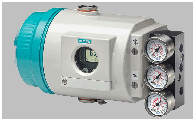
SIPART PS2 in flameproof aluminum enclosure (Ex d) with gauge block (optional)
