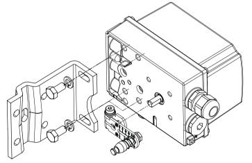
Figure 4-5 Installation with mounting bracket
